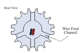
**Note:** There are four lateral wire feed channels cut into the rear of the LED fixture. The wires can be run through one and set flush to the mounting surface. No wire hole would be drilled under the light.
